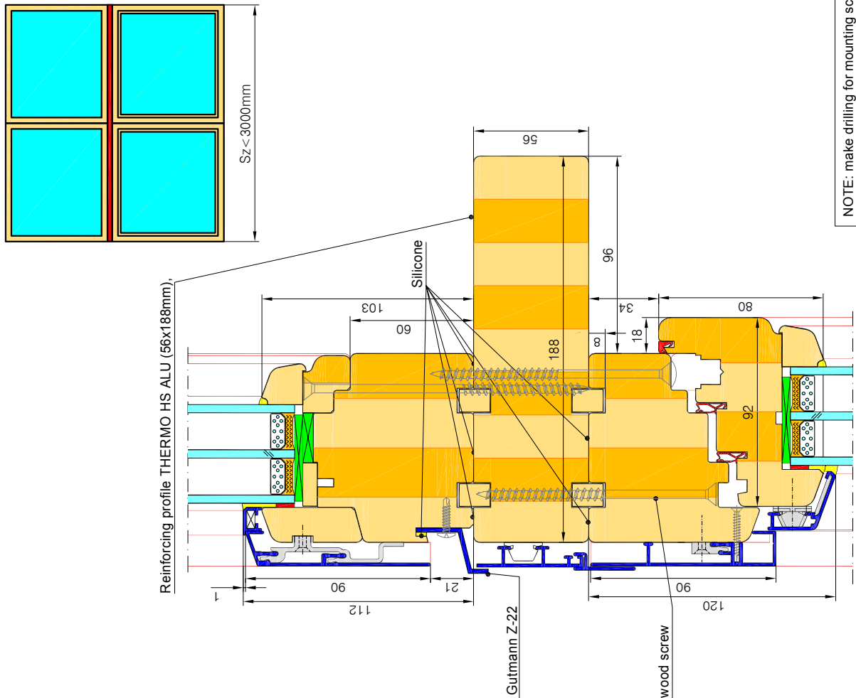
Reinforcing profile for window set 188 x 56mm.
